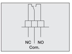
NC: normally closed Com: common NO: normally open
